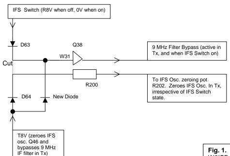
**Fig. 1.** Electrical schematic of the W2ISB Passband Tuning Modification for the Icom IC-765
